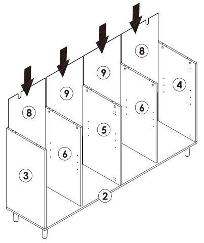
Insert panels 8&9 downwards along the pull groove
