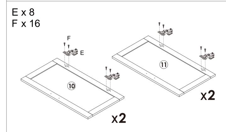
Lock hardware accessory E onto panels 10&11 with screws F.
