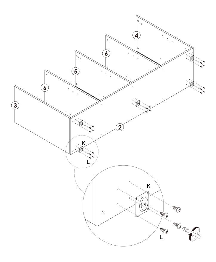
Connect hardware K to panel 2 with screw L.
