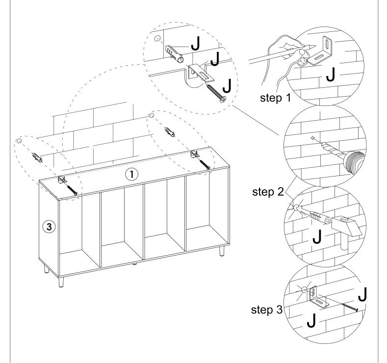
If it is a solid wall, please use expansion and self-tapping screws to secure the cabinet to the wall, if it is a wooden wall, only use self-tapping screws. Please don't overtighten screws.
