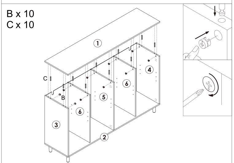
the slot of panels are downward. connect panel 1 to panel 3&4&5&6 with hardware B and C.
