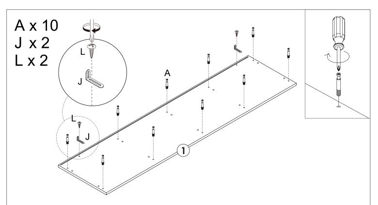
screw A to panel 1, connect hardware J to panel 1 with screw L. Screwdrivers are not included in the accessories.
