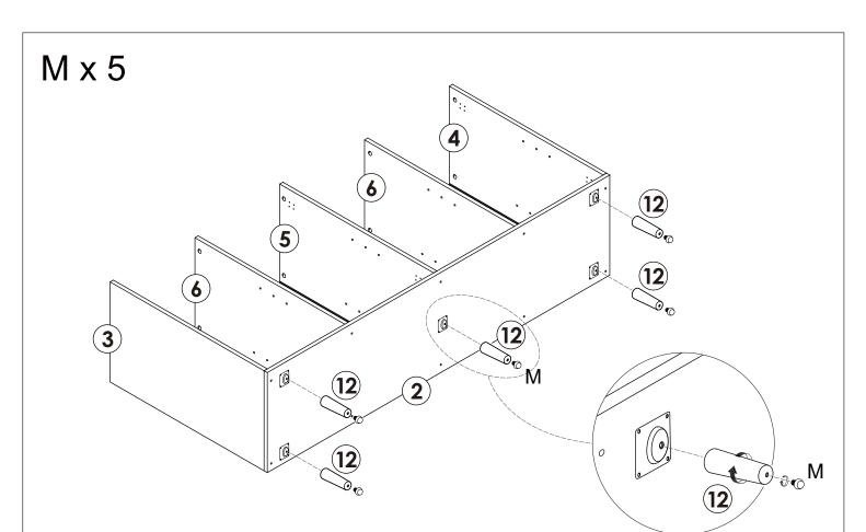
Screw hardware accessory M onto plate 12. Screw plate 12 onto accessory K again.
