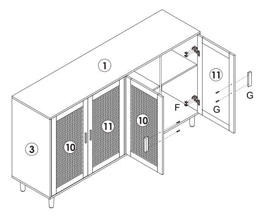
Lock hardware accessory G onto door panels 10&11. Lock door panels 10&11 onto panel 4&5 using screws F.
