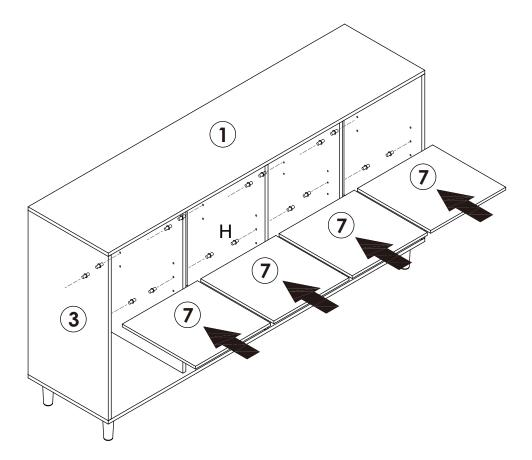
Insert hardware accessory H into the holes of partitions 3&4&5&6.
