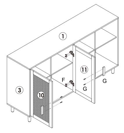
Lock hardware accessory G onto door panels 10&11. Lock door panels 10&11 onto panel 3&5 using screws F.
