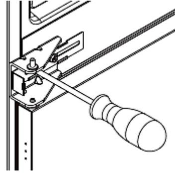
6. Unscrew the top hinge pin. Turn the hinge and reinstall the hinge pin.
