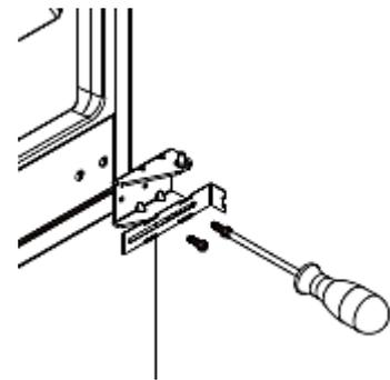
3. Move the bottom hinge pin from the right to the left side.
