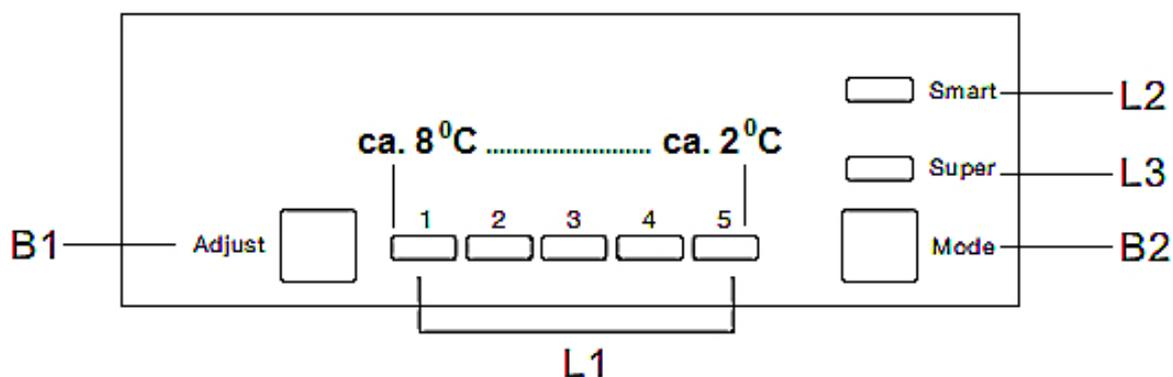
The power levels [ 1 – 5 ] regulate the different values of the internal temperature.
