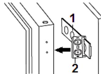
7. Check that the doors can be closed and opened smoothly and properly. Check that the door seals close properly. If not, slightly adjust the appliance. Then fix the bottom bracket on the cabinet using two long screws.
