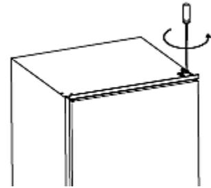
2. Unscrew the middle hinge. Remove the bottom door and store it in a safe place so it cannot be damaged.
