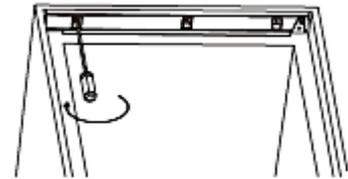
9. Seal the gap between the appliance (door-opening side) and the cabinet using the sealing tape.
