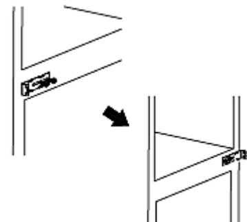
5. Move the middle hinge to the left side. Before you tighten the middle hinge, ensure proper horizontal and vertical position of the bottom door so the door seals will close properly.
