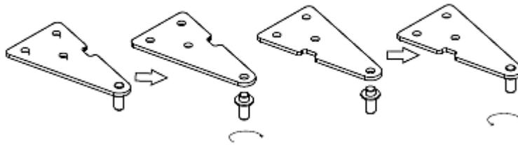
7. Fit in the top door. Move the top hinge to the left side. Before you tighten the top hinge, ensure proper horizontal and vertical position of the top door so the door seals will close properly.
