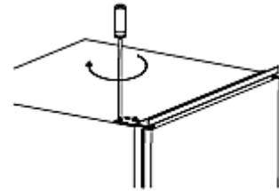
**NOTICE! Adjust the doors properly. The seals must close properly.**
