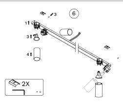
Fix base into place, apply side screws, insert the bulbs by rotating & tie up the caps
