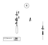
Apply anchors & tie up screws to install the base on the ceiling
