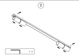
Untie side screws & secure canopies into steady position
