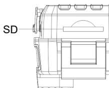
Note: The camera does not have a built-in memory, so a memory card must be inserted into the camera before use. If the memory card has been used in a different camera, format the memory card in the wildlife camera before use.
