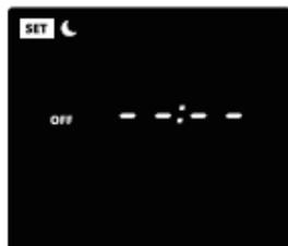
**OFF:** The night mode is disabled. In the event of inactivity for a longer period, the display and the LED indicator light always remain switched on.
