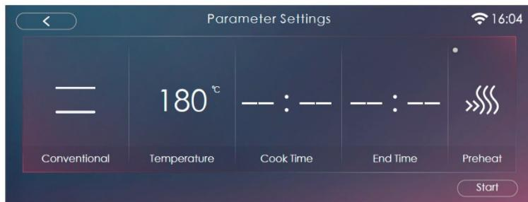
You can combine the cooking time and finish time functions to specify the desired on and off time of the oven. This allows you to program the cooking function while you are away, or the defrosting function ready for you to cook when you return home.
