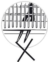
When loading the cutlery, ensure that it does not protrude through the bottom of the cutlery basket. Otherwise, the lower spraying arm will be blocked.
