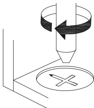
**EN**\_Turn cam lock clockwise to tighten.
