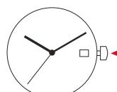
Pull crown all the way out and turn to correct time. Push crown in to restart.
