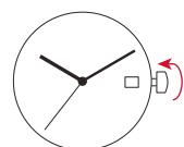
For screw-in setting crown, turn COUNTERCLOCKWISE to loosen.
