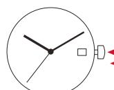
For screw-in setting crown, push crown in while turning CLOCK-WISE to tighten.
