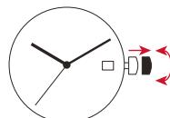
**2-Position Crown:** Pull crown to "OUT" position and turn CLOCKWISE until date changes. Repeat until correct date appears. Adjust date when month has less than 31 days. Push crown in when finished.
