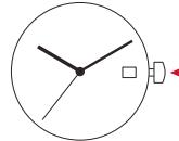
Press button or crown to activate light. Patented electroluminescent technology is used to illuminate the entire watch face at night and in low light conditions.
