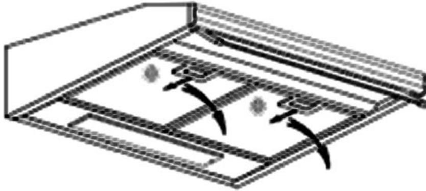
After removing the small plastic plate / cover<sup>3</sup> you (optionally) can install the adapter. Insert the exhaust hose into the adapter.
