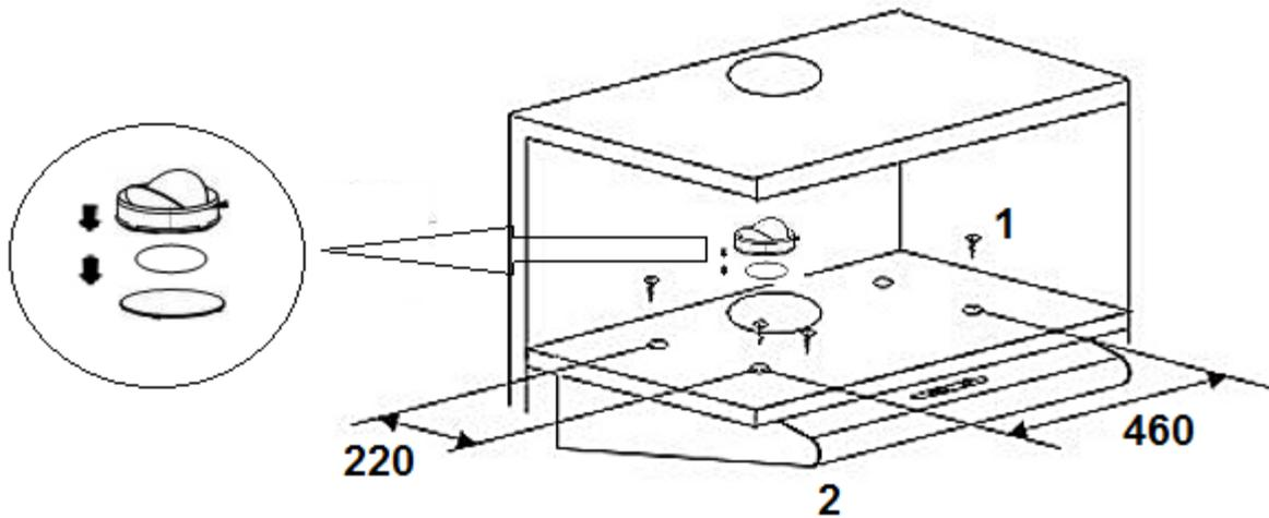
1. Drill four holes ( $\text{Ø } 4 \text{ mm}$ ) in into the bottom of the cupboard.
