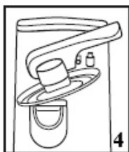
When the can is fully open, the cutting action will automatically stop. The can will remain in position until the lever is raised.
