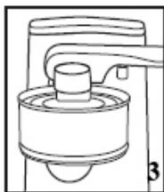
Push the can opener lever down firmly and hold until the can lid is automatically pierced and the cutting action begins as shown in figure 3.
