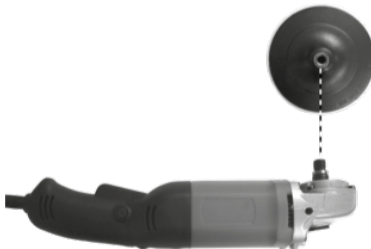
Figure 2: Installation of polishing plate
