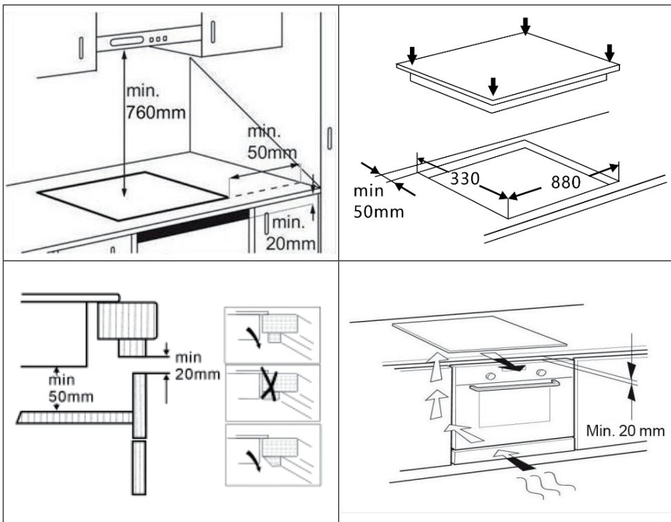
**Note:** The distance between the underside of the appliance and the separator panel must respect the dimensions given in the figure (min. 50 mm).
