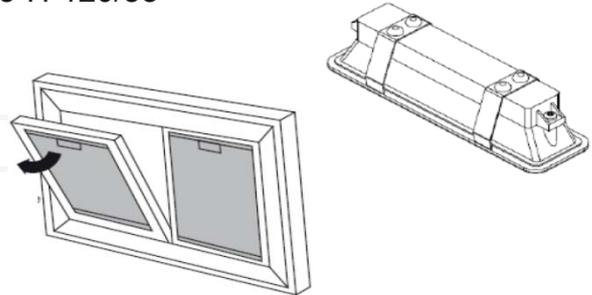
3 Press the lamp module out of the hood housing from the inside.
