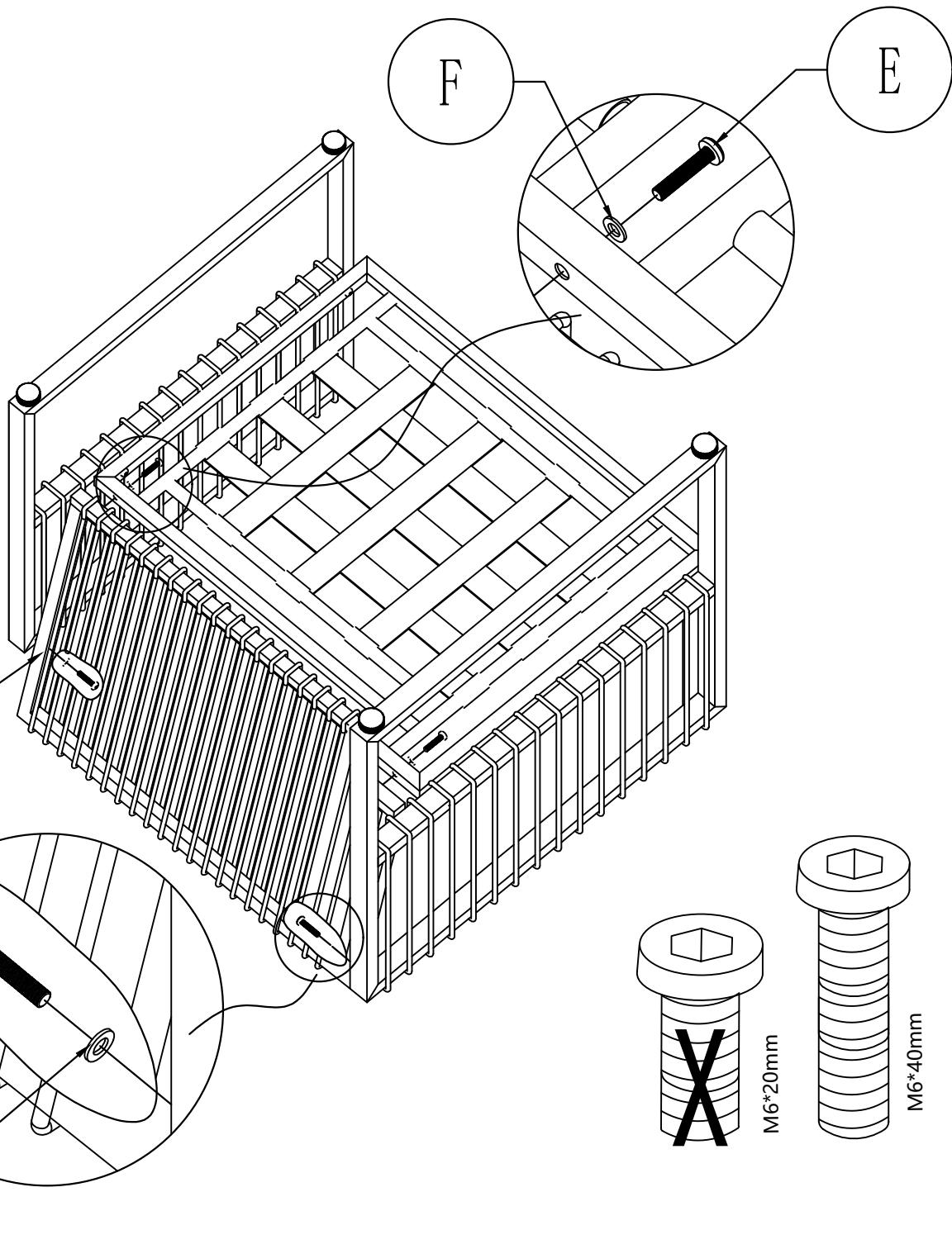
**EN:** Connect back (K) & right arm(B) & left arm (C)&seat (A)with Bolt (E), Washers (F) .
