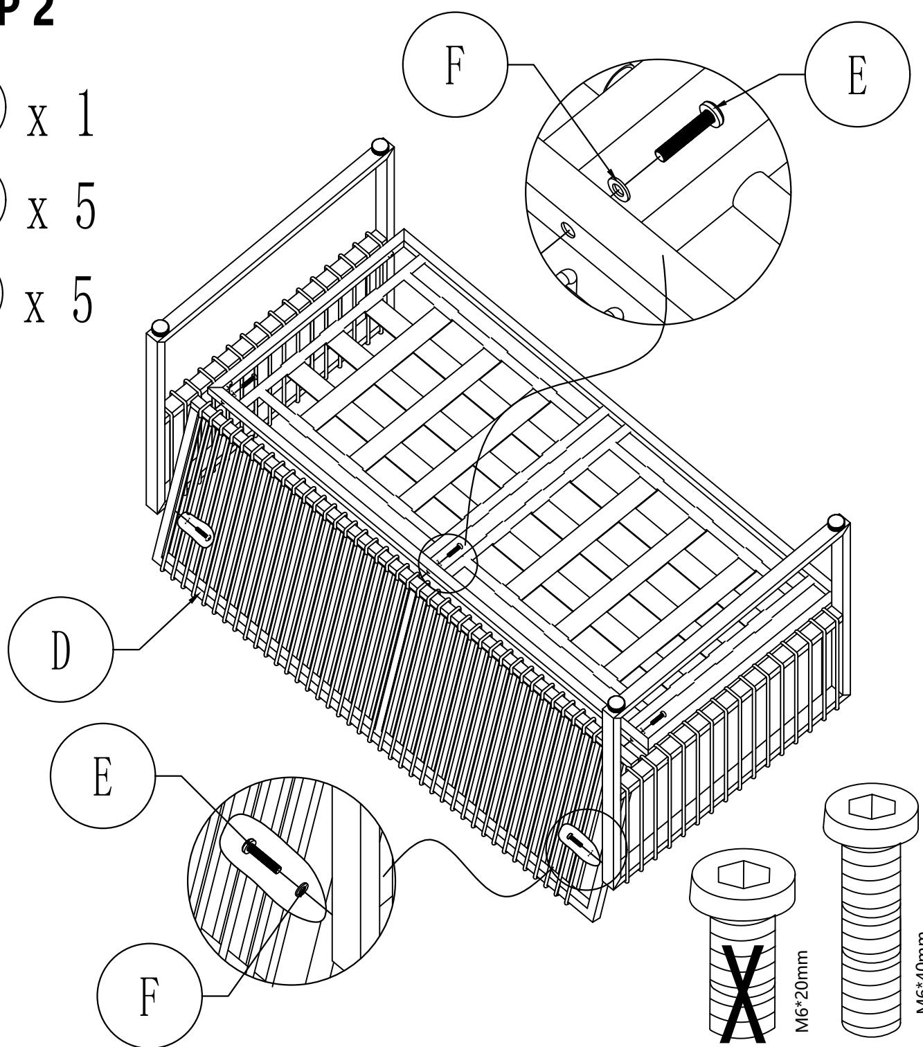
**EN:** Connect back (D) & right arm(B) & left arm (C)&seat (A)with Bolt (E), Washers (F) .
