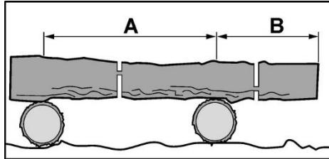
**Important:** Do not saw logs that are under tension! Splintering wood or a tilted saw-bar can cause serious injuries!
