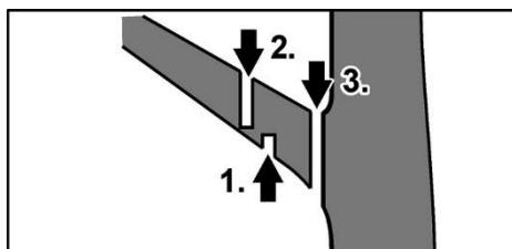
**Caution:** Branches that are resting or under tension can wedge the saw-chain in the wood!
