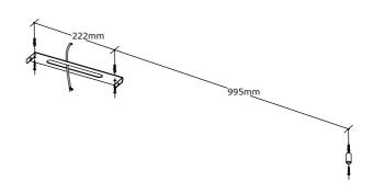
2. Align, Mark and drill holes to apply the screws
