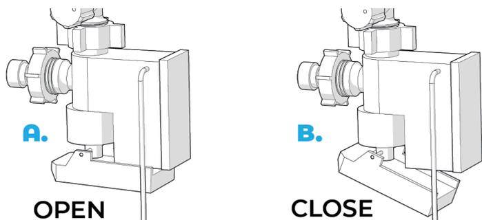
After this test, please close the switch flap again in position **A.** Thoroughly dry the sensor and then place it back on the floor.
