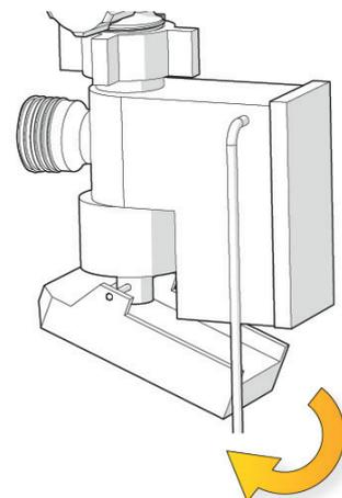
After successful installation of the Hydro-Stopper, please connect the chosen household appliance to the Hydro-Stopper outlet, which has a 3/4" external thread. If your device has a different type of connection, we recommend purchasing an appropriate adapter, as such an adapter is not included in the installation kit due to the variety of connections.
