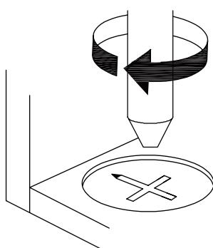
**EN**\_Turn cam lock clockwise to tighten.
