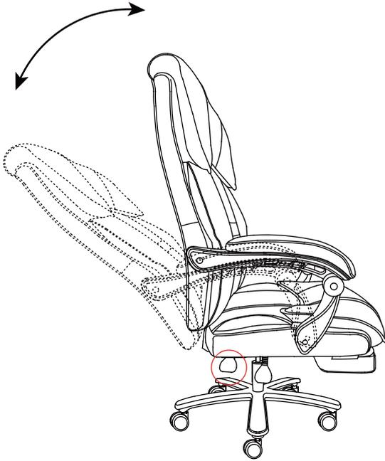
*Pull the lever FULLY and lean back slowly until desired angle is achieved, then slowly return the lever to its starting position. Ensure the lever locks back in place.*
