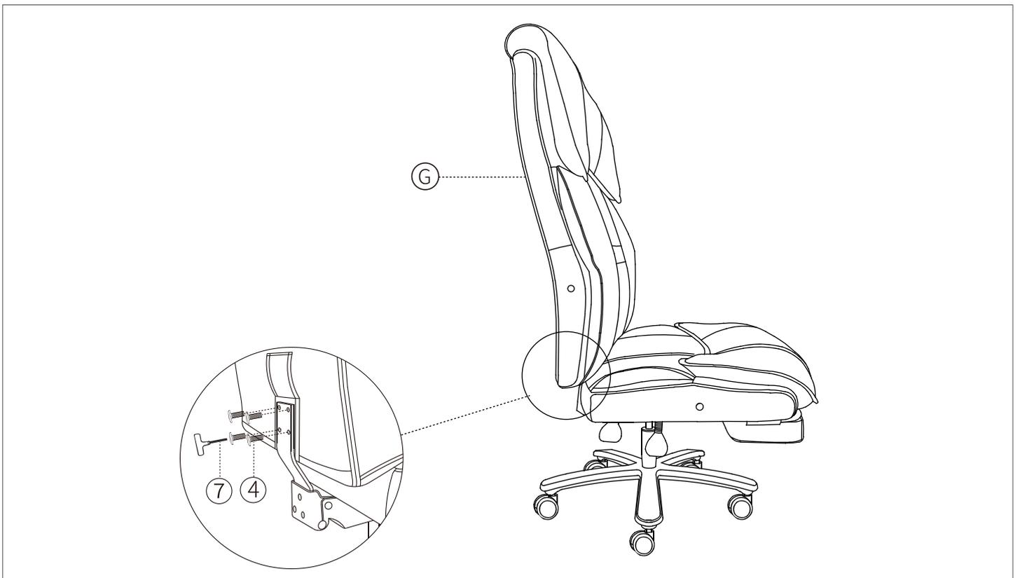
**STEP 7:** Attach armrest to the connector with M8\*45mm Bolts on both sides, using the T-Wrench.
