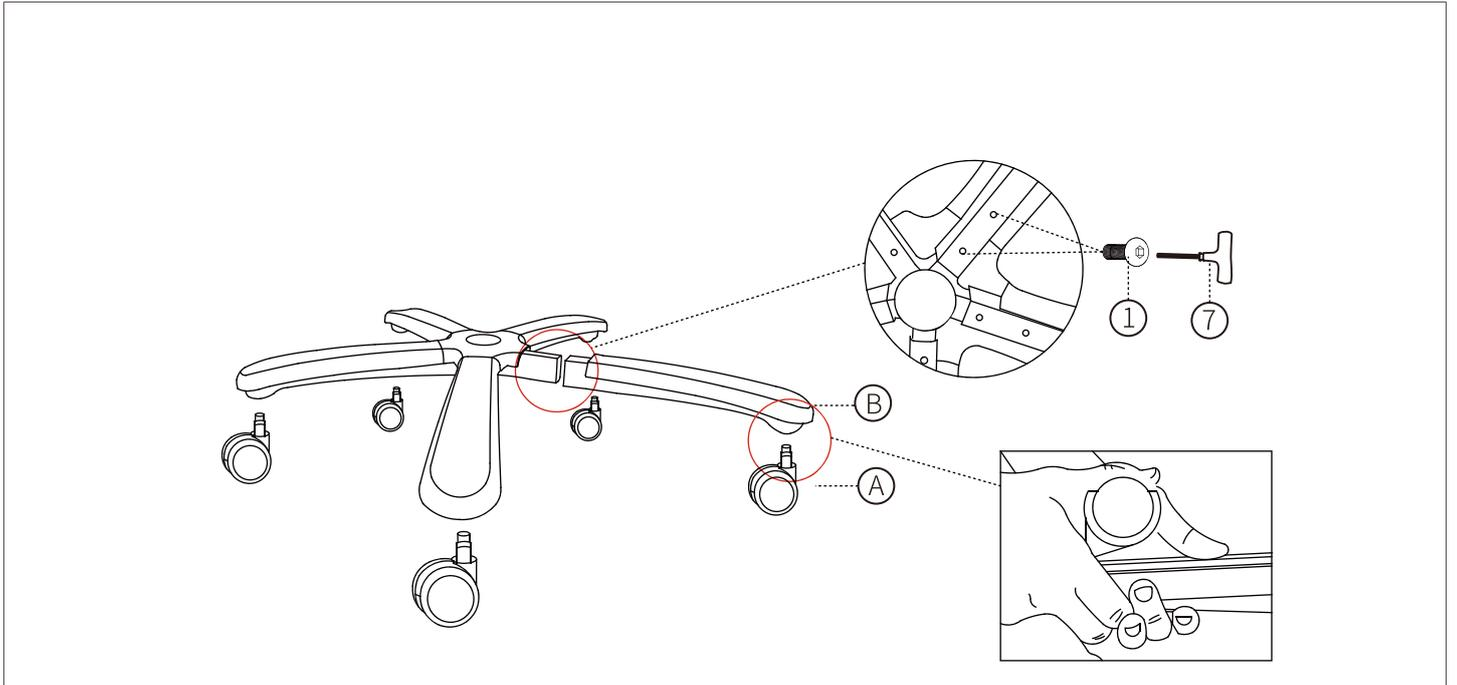
**STEP 2 :** Turn the Star Base upright and insert the Lift into the center hole of the Star Base.
