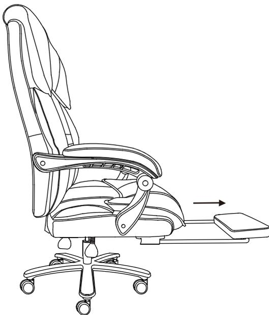
*Pull out the pole of the footrest, and turn the footrest to the front.*
