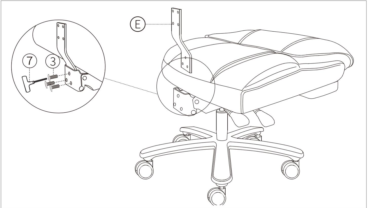
**STEP 6:**Attach the Steel Plate to the back cushion with four M6x25mm Bolts.
