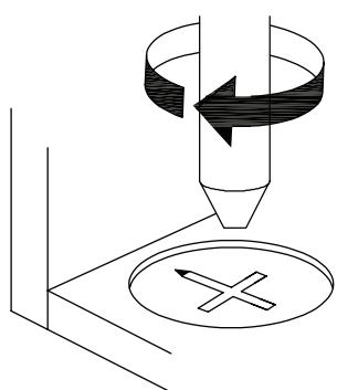
**EN**\_Turn cam lock clockwise to tighten.
