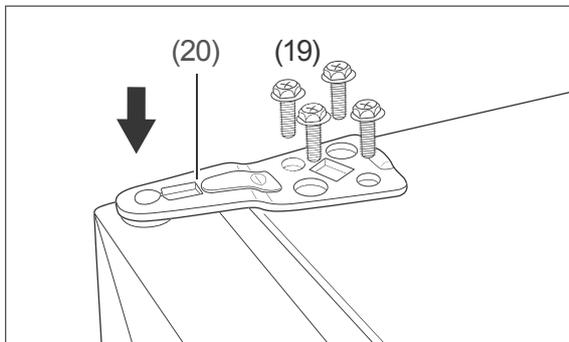
5. Tighten the upper hinge (20) with the screws (19).
