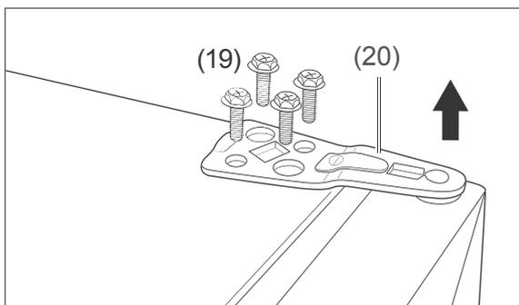
4. Ensure that the glass door cannot slip away (1) and loosen the screws (19) on the upper hinge (20). Use the cross-tip screwdriver.
