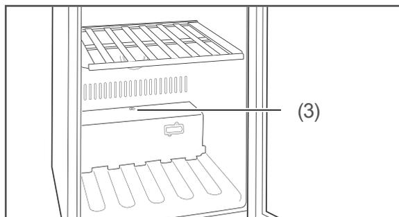
8. Clean the opening of the thaw water drain (3) using a cleaning rod.
