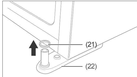
7. Remove the washer (21) from the lower hinge (22).
