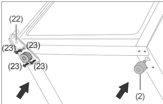
1. Tighten the lower hinge (22) on the other side using (23) the screws.
