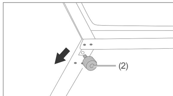
9. Remove the screw foot (2) and screw it back in on the opposite side.
