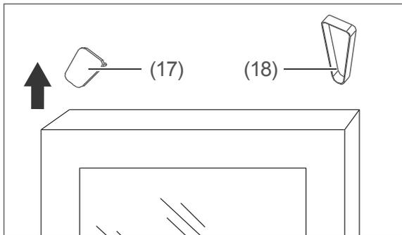
3. Gently push the blanking plate (17) and hinge cover (18) upwards with a slotted screwdriver and remove them. Hold onto the blanking plate and hinge cover.
