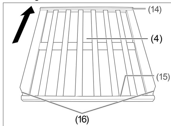
1. Turn the bottle shelf (4) so that the front rail (15) and back rail (14) are facing up and the chamfered edges (16) are facing forward.
