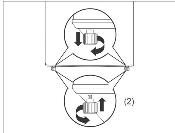
4. Level out any unevenness on the ground using both of the front screw feet.
