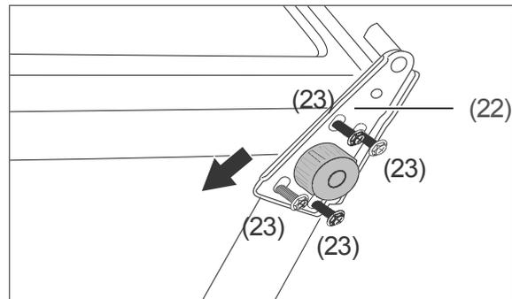
8. Loosen the screws (23) and remove the lower hinge (22) from the appliance.
